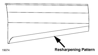
Do not sharpen to original pattern (below). It is easier to get a straight cutting edge following the resharpening pattern shown above.
